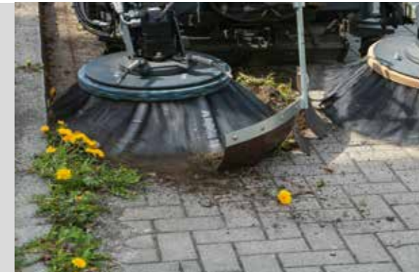
Chemical-free against weeds: with a weed broom for mechanical removal and collection of weeds.
