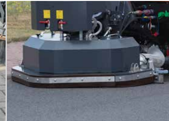
Wet cleaning made easy: the scrubbing deck removes even stubborn dirt from smooth surfaces.
