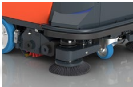
Cylindrical brush and side broom enable wet cleaning and sweeping in a single working step.
